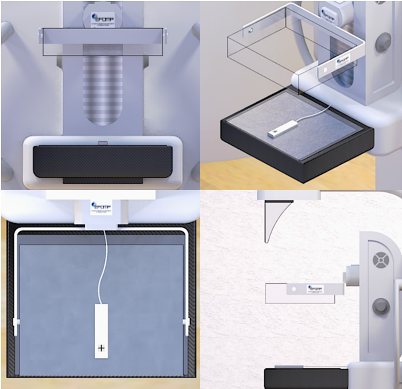
Figure 30 Schematic showing the setup for the measurement of K_m .
