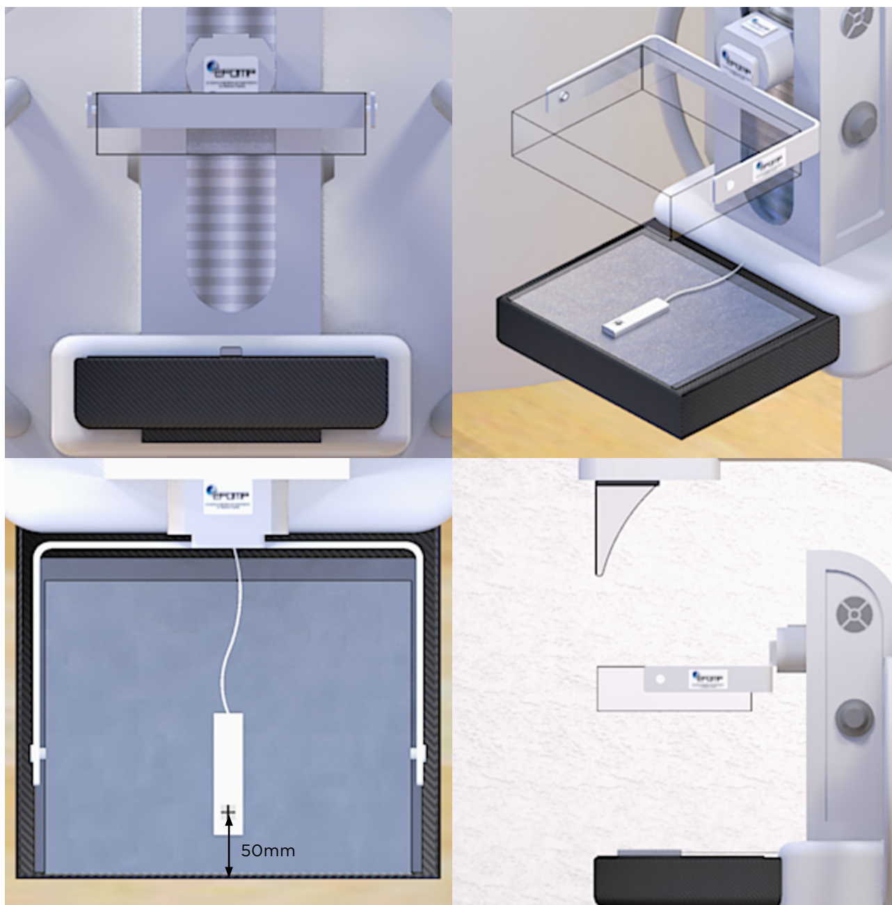
Figure 1 Setup for the HVL measurement using a calibrated x-ray multimeter
