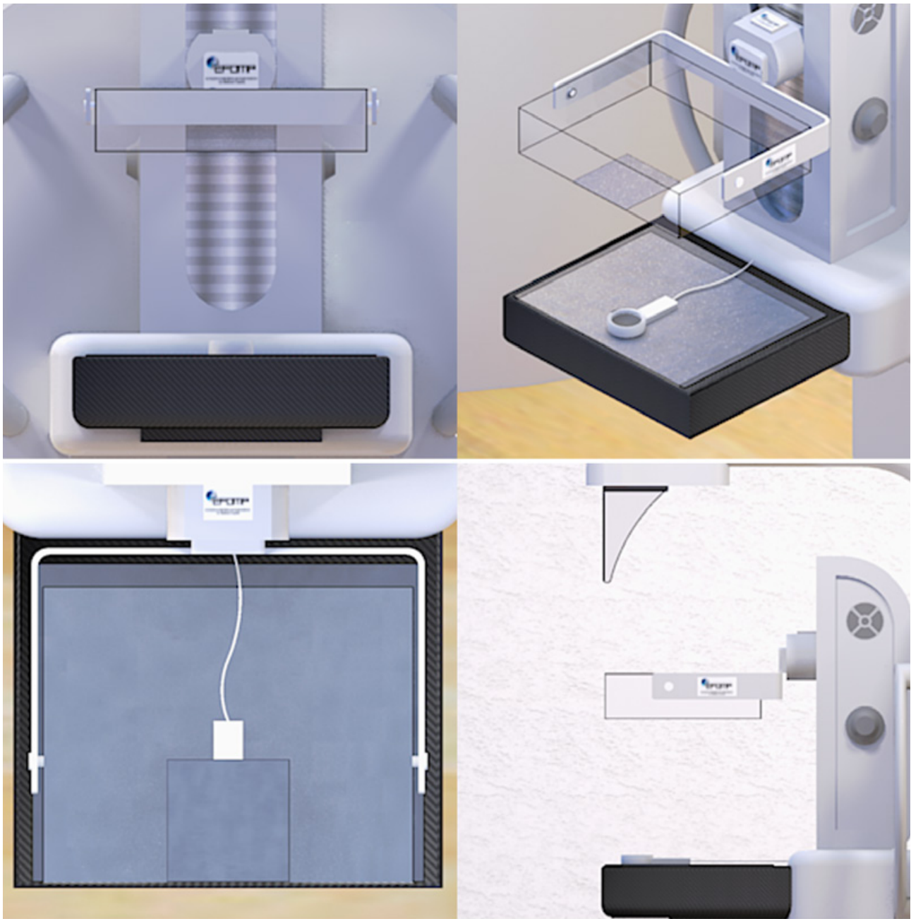
Figure 2 Setup for the HVL test using ion chamber and aluminium filters
